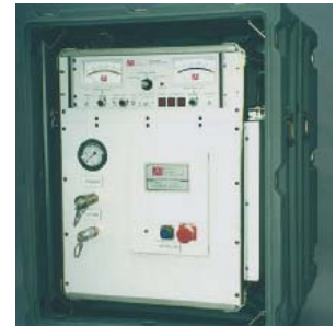
Field Test Hydraulic Power Supply
