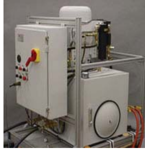
Water Cooled Laboratory Hydraulic Power Supply
